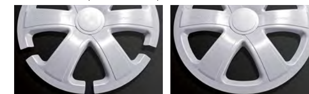
The FFC molding enables complete filling without raising injection pressure.
