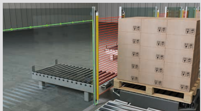
Smart Process Gating on a conveyor line
