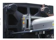
control under high injection pressures; selectable force settings for compatibility with various mold types (hot runner, cold runner, floating sprue bushings, etc.); and rapid pressurization/depressurization for faster cycle times.
