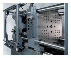
All SEEV-A model sizes were designed with ample tie bar space, in a square configuration, to accommodate larger side-entry molds.
