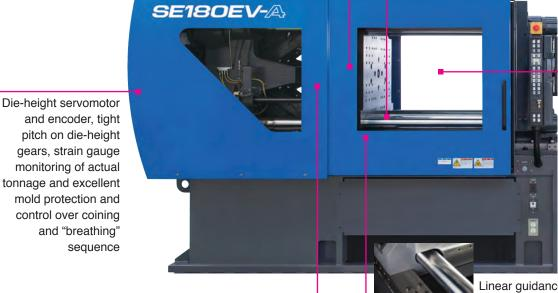
Fast clamp open/close speeds up to 47.2 in/s (1200 mm/s) plus new S-MOVE technology that optimizes the mold open/close speed pattern, decreasing vibration and cycle times
