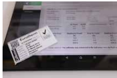
With the eCAT tool, an instrument test produces a certificate and QR label
