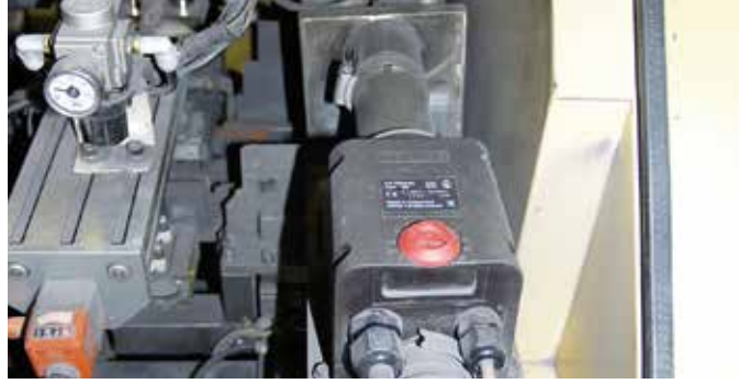
Deflashing foil sleeves from charcoal filter elements
