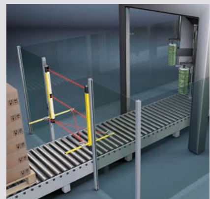
Timing controlled 2-sensor muting
