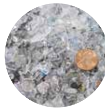
PET Flake w/Aluminum (4mm-10mm) 96% Aluminum Contamination Removed
