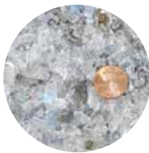
PET Flake w/Aluminum (<4mm) 93% Aluminum Contamination Removed
